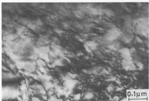
Figure 3 Evidence for the formation of proeutectoid ferrite in a 9Cr–1Mo–0.07C steel austenitized at 1323 K and air cooled.
